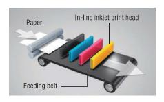
Instand-drying ink complements the high-speed, duplex printing capability. This specially developed, oil-based ink is also fade resistant and water resistant and minimizes paper cirling. Stable paper feeding ensures the reliable performance necessary for high speed printing.
